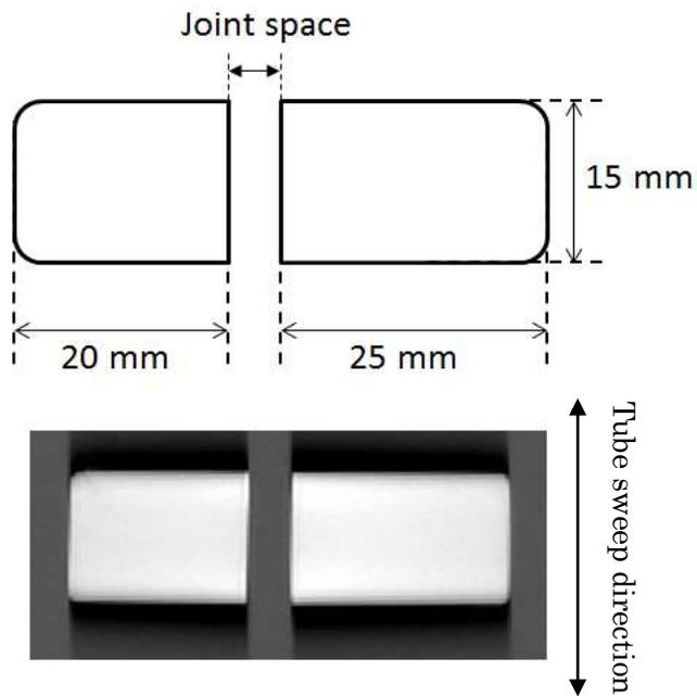
Fig 5 Image with illustration of joint space phantom.
