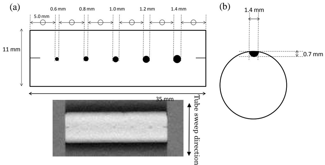
Fig 1 Detailed sizes of bone erosion phantom.
