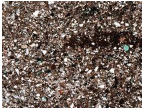
Fig. 1 Thin sectional image of the sandstone at 180 m deep of the drill hole at 650 m of #2 inclined shaft (the width of the image is 3.5 mm, Matsumoto et al., 2014)
