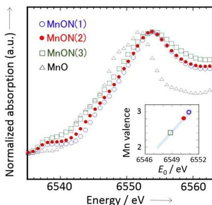
**Figure 3.** X-ray absorption  $K$ -edge of manganese oxynitrides. Inset shows the calibration line for the estimation of Mn valence from inflection points ( $E_0$ ) using MnO and  $\text{Mn}_2\text{O}_3$  standards.
