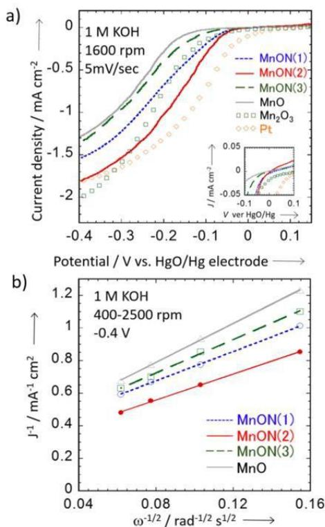
**Figure 4** a) Linear sweep polarization of MnON(1), MnON(2), MnON(3), and MnO with rotating disc electrode in  $\text{O}_2$ -saturated 1 M KOH solution at a sweep rate of  $5 \text{ mV sec}^{-1}$ . Polarization of Pt/C and  $\text{Mn}_2\text{O}_3$  is shown for comparison. b) Koutecky-Levich plots at  $-0.4$  eV with rotation speeds of 400-2500 rpm.
