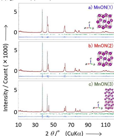
**Figure 2.** Rietveld profiles of X-ray diffraction of a) MnON(1), b) MnON(2), and c) MnON(3). Bars indicate the calculated positions of Bragg peaks and bottom lines represent residuals. Insets show cell structural models: large and small spheres represent Mn and O/N sites, respectively. Lines represent unit cell boundaries and the Mn<sub>4</sub>(O,N)<sub>4</sub> cell.
