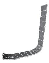
Figure 5.4: Retractor model. The white spheres are the vertices of the surface polygons, which used to detect the penetration with deformable models. The number of vertices and faces are 712 and 1352, respectively.
