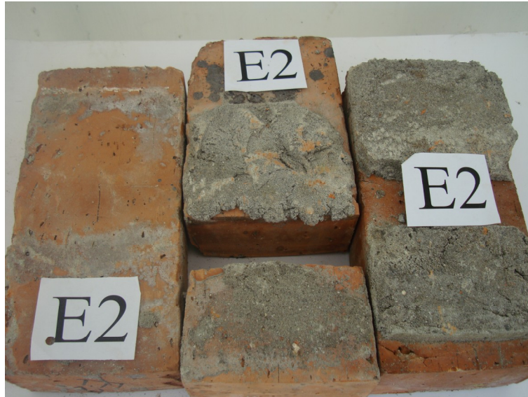
Fig. 3.9. Failure surface of a typical shear specimen
