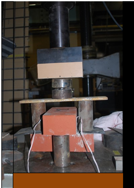
Fig. 3.14. Experimental setup of crossed-brick test
