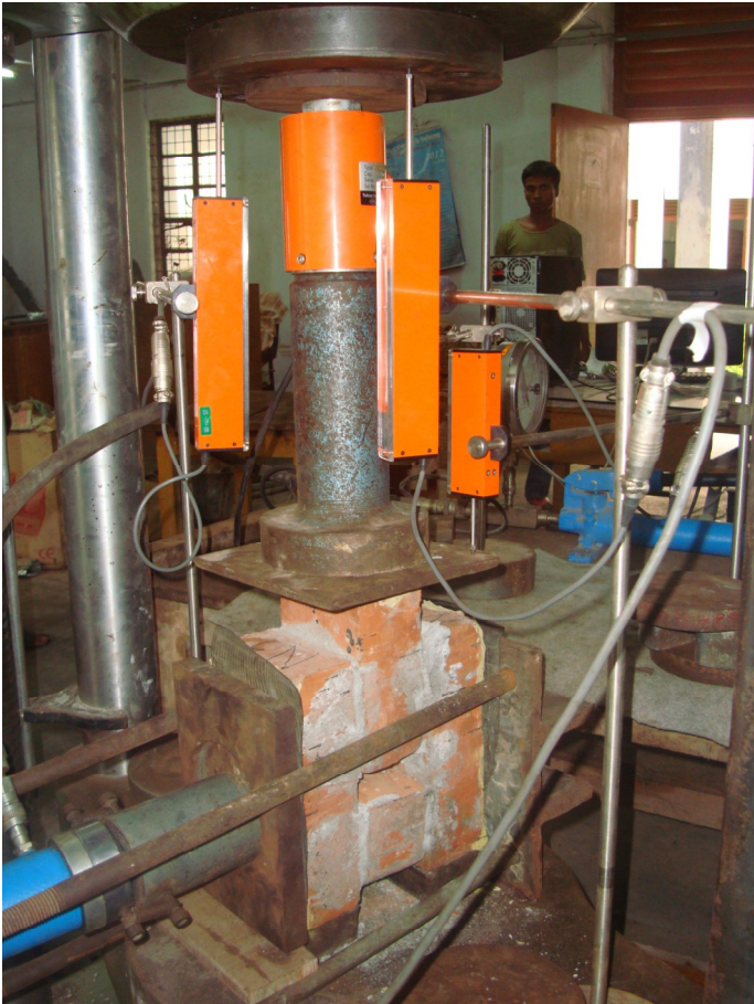
Fig. 3.4. Instrumentation and test setup of shear specimen
