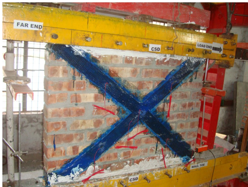
Fig. 5.13. Experimental setup of FRP reinforced masonry
