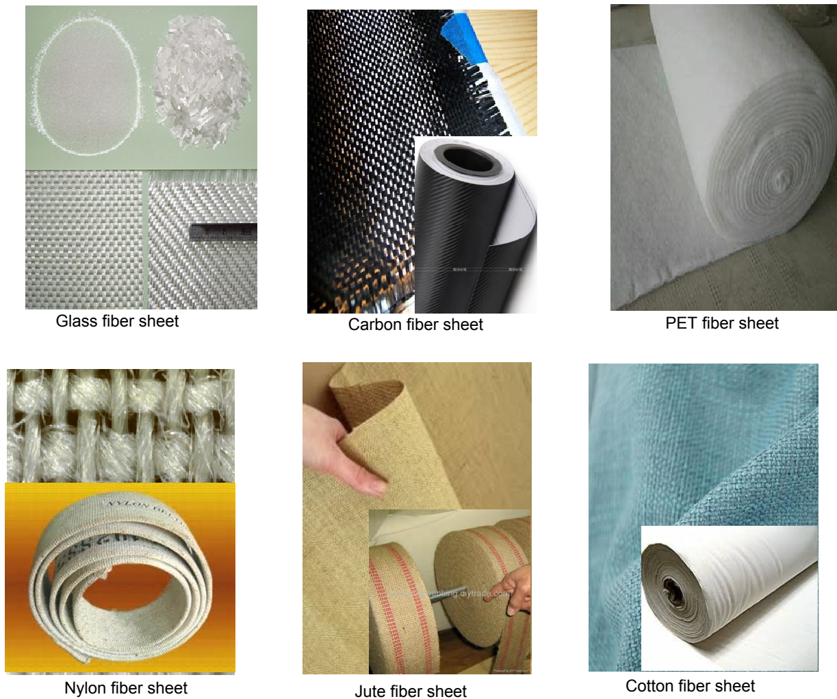
Fig. 2.9. Common types of fiber sheet (NGCC, 2008)
