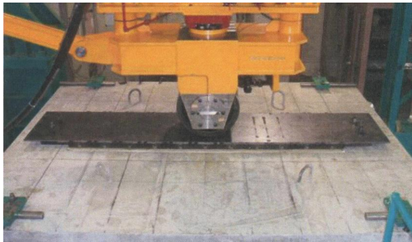
Fig. 1.5 Moving load test
