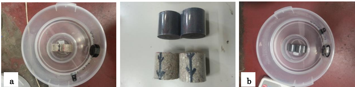
Fig. 3 Jacketed samples in air-tight containers with pure water (a) arkose sandstone (b) fine-grained sandstone.
