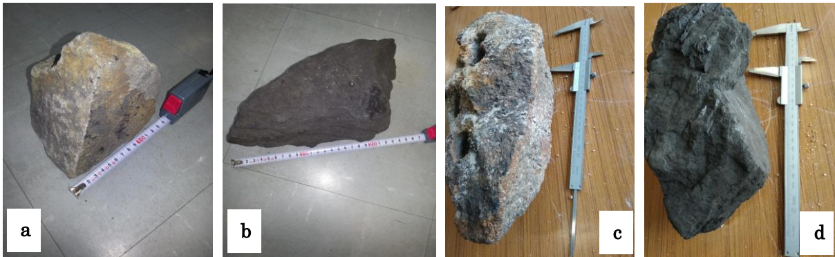
Fig. 1 Rock samples from Mchenga coal mine (a) arkose sandstone (b) fine-grained sandstone; and Kaziwiziwi coal mine (c) arkose sandstone (d) fine-grained sandstone
