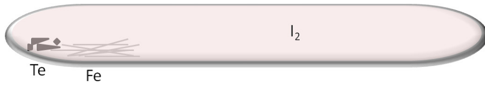
Figure 2.1: Schematic view of ampoule used for the chemical vapor transport with using iodine as the transport agent.
