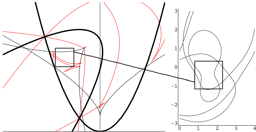
Figure 3. Beaks: two regular parts of the CS become tangential.
