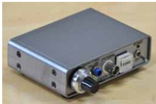
Fig.2.23 Elevator machine control device
