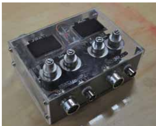
Fig.2.10 Amplifier of rudder dynamometer
