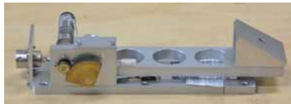
Fig.2.22 Elevator machine for prism
