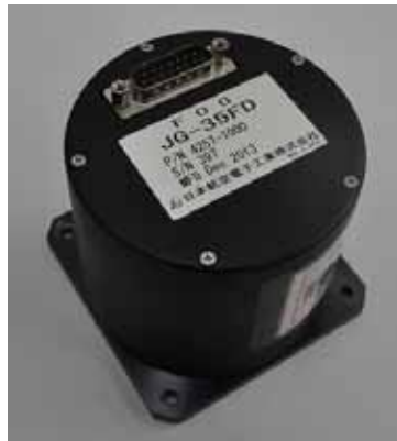
Fig.2.12 Fiber optic gyro
