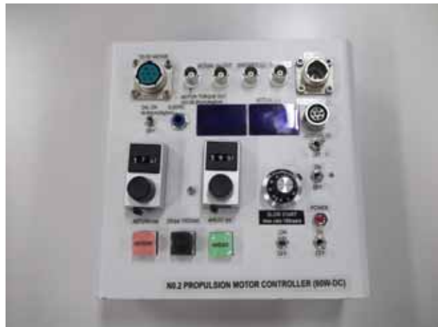
Fig.2.6 Motor control device
