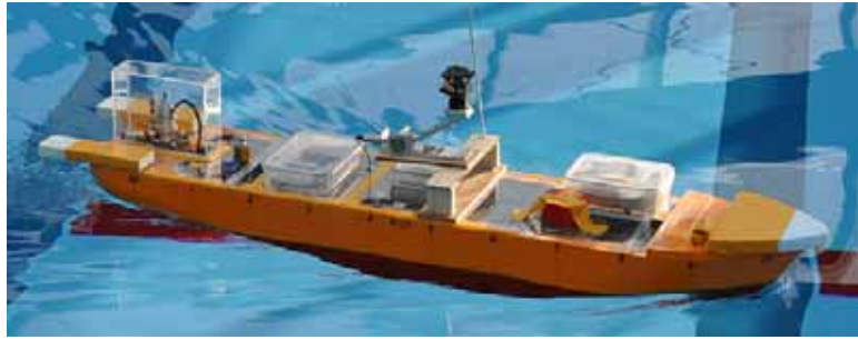
Fig.2.24 Arrangement of model ship with all devices
