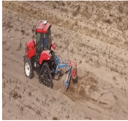
Fig.2. 24 Building bumps and hollows using a plough
