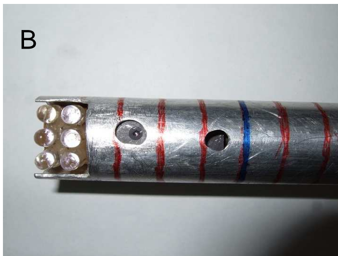
Photo 1 A cavity measurement system. A cavity viewer using a wireless CCD camera was originally developed by Matsuoka (2002; 2010).
