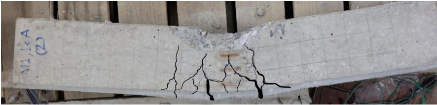
Figure 3.12. Crack formation of non-damaged beam strengthened with method 1 in combination with SPCM_PE
