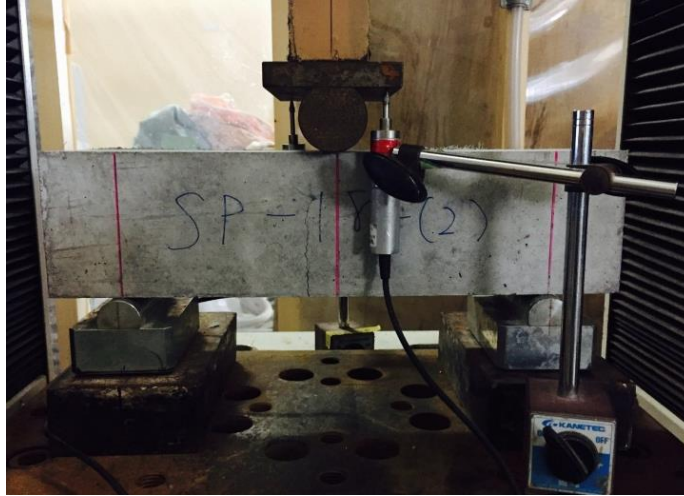
Figure 2.3: Three point bending test setup
