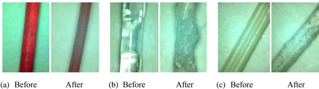
Figure 2.11: The fiber surface before and after the flexural test. (a) R-Nylon fiber; (b) R-PET fiber; (c) PVA fiber (30 mm)
