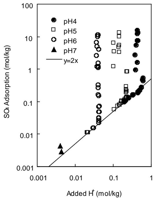
**Fig. 1.** Sulfate adsorption and added protons to maintain constant pH in the adsorption experiment. A H<sub>2</sub>SO<sub>4</sub> solution was added for the pH adjustment.
