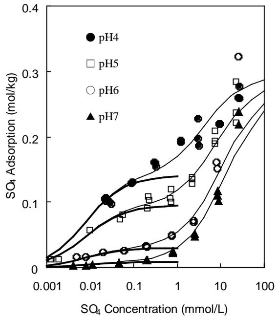
**Fig. 5.** The measured sulfate adsorption isotherms and the calculated Langmuir isotherms. The thick lines were obtained using Eq.(4). The thin lines were obtained using Eq.(6).
