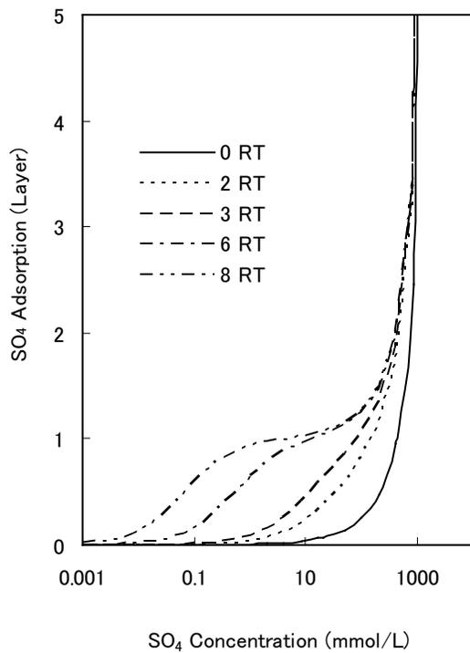
**Fig. 3.** The calculated BET isotherms. Values for the lines denote the binding energy difference between the monolayer and the other layers,  $\Delta\varepsilon = \varepsilon_S - \varepsilon_L$ , as expressed in Eq.(2). The unit in the ordinate, Layer, indicates the covering ratio of sulfate on the soil surface.
