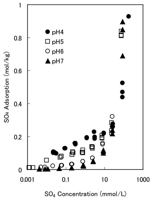
**Fig. 2.** Measured sulfate adsorption isotherms.
