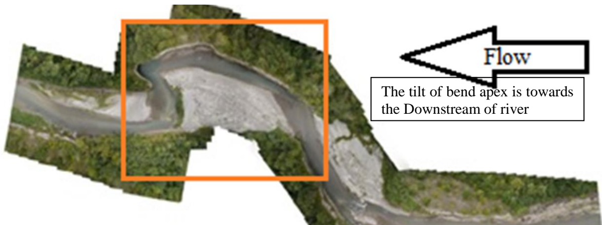
Figure.5.2 Meandering Shikaribetsu river. It is a bedrock river in Hokkaido, Japan. Image courtesy: Takuya Inoue
