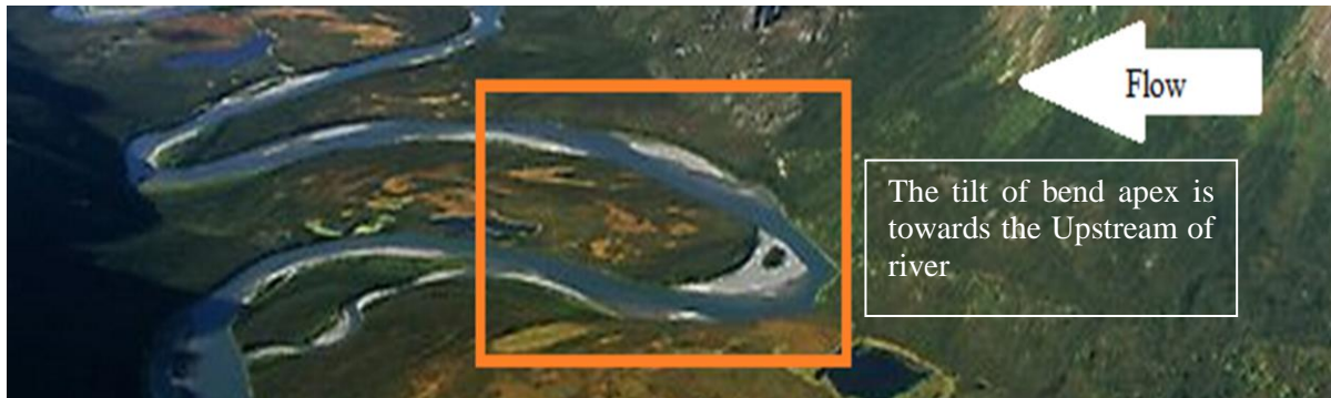
Figure.5.1 Kinoshita type meandering in Atlanta river, Alaska, USA. Image courtesy: Google Images
