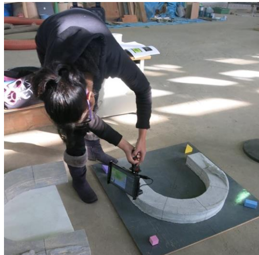
Figure 2.6 Obtaining 3D scan of the mold
