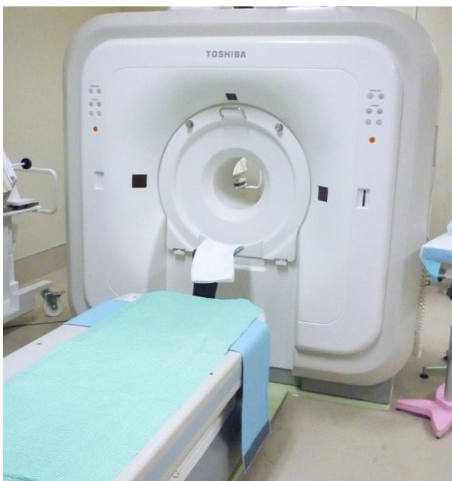
Figure 7. SPECT. SPECT data were acquired using a triple-head gamma camera (GCA-9300/DI, TOSHIBA, Tokyo, Japan).
