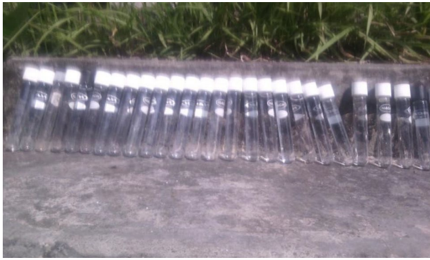
Fig. 1 Solar irradiation of water samples in the presence of \text{Fe}_2\text{O}_3 NPs
