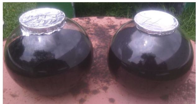
Fig. 2 Solar irradiation of textile wastewater samples in the presence of \text{Fe}_2\text{O}_3 NPs for irrigating on plants
