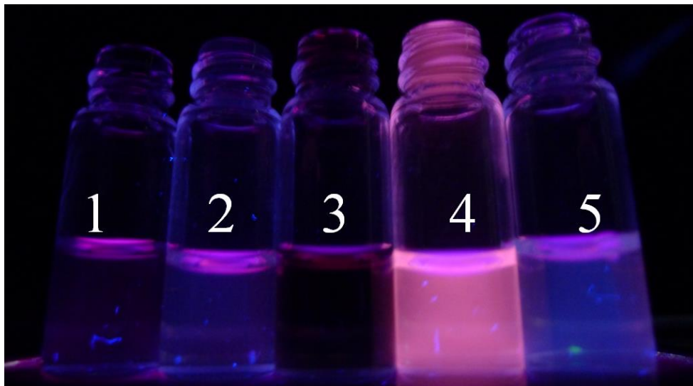
Figure S3. Color of the solution of monometallic plasmonic nanoparticles: (1) Au@20mA, (2) Ag@34mA and its corresponding plasmonic alloy nanoparticle (3) Au@20mA-Ag@34mA and monometallic photoluminescent nanoclusters synthesized with MUTAB: (4) Au@20mA and (5) Ag@34mA under UV-light irradiation.
