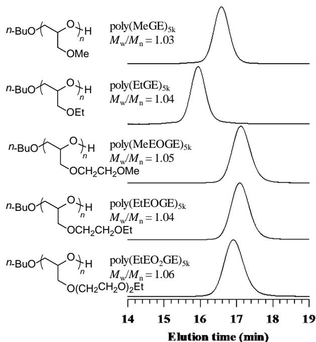
**Figure 1.** SEC traces of poly(MeGE)<sub>5k</sub>, poly(EtGE)<sub>5k</sub>, poly(MeEOGE)<sub>5k</sub>, poly(EtEOGE)<sub>5k</sub>, and poly(EtEO<sub>2</sub>GE)<sub>5k</sub> (eluent, THF; flow rate, 1.0 mL min<sup>-1</sup>).
