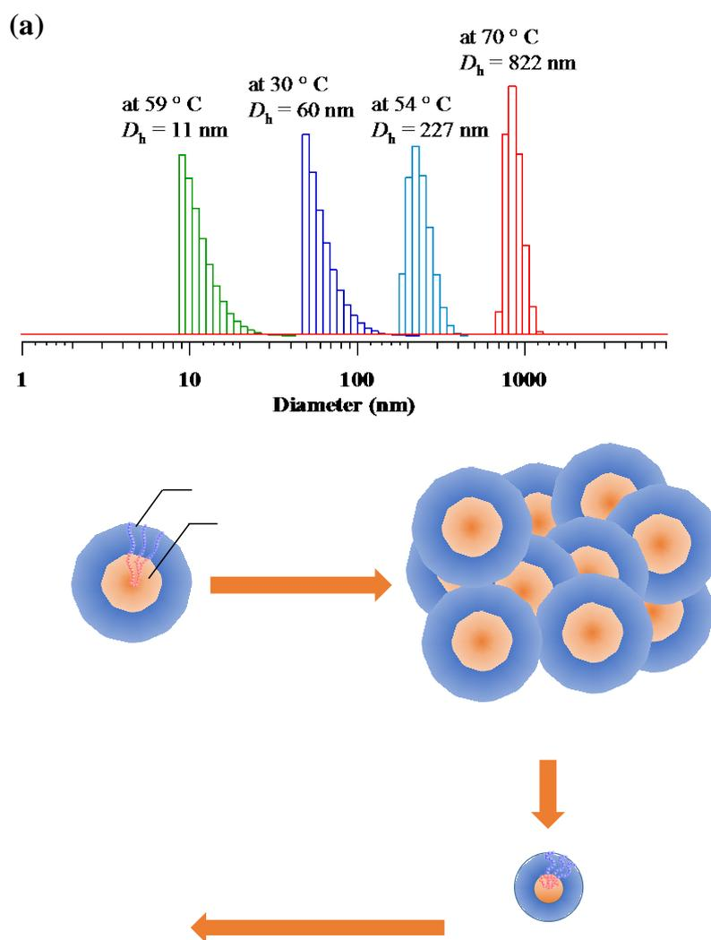
**Figure 9.** (a) Number-average particle size distributions for the aqueous solution of poly(MeEOGE<sub>0.50</sub>-*b*-EtEOGE<sub>0.50</sub>)<sub>14k</sub> at 30, 54, 59, and 70 °C determined by DLS. All the measurements were performed using a 1 wt% aqueous solution. (b) Possible mechanism for the complexed phase behavior observed in the aqueous solution of poly(MeEOGE<sub>0.50</sub>-*b*-EtEOGE<sub>0.50</sub>)<sub>14k</sub> upon heating.
