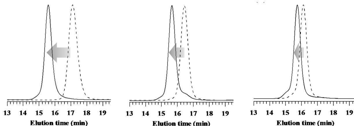
**Figure 7.** SEC traces of (a) poly(MeEOGE<sub>0.24</sub>-*b*-EtEOGE<sub>0.76</sub>)<sub>18k</sub>, (b) poly(MeEOGE<sub>0.50</sub>-*b*-EtEOGE<sub>0.50</sub>)<sub>14k</sub>, and (c) poly(MeEOGE<sub>0.75</sub>-*b*-EtEOGE<sub>0.25</sub>)<sub>14k</sub> (eluent, THF; flow rate, 1.0 mL min<sup>-1</sup>). The broken lines indicate the poly(MeEOGE)s prepared by the first
