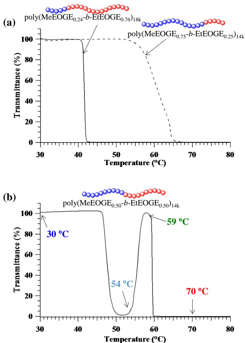
**Figure 8.** (a) Transmittance curves for the 1 wt% aqueous solutions of poly(MeEOGE<sub>0.24</sub>-*b*-EtEOGE<sub>0.76</sub>)<sub>18k</sub> (solid line) and poly(MeEOGE<sub>0.75</sub>-*b*-EtEOGE<sub>0.25</sub>)<sub>14k</sub> (broken line). (b) Transmittance curve for the aqueous solution of poly(MeEOGE<sub>0.50</sub>-*b*-EtEOGE<sub>0.50</sub>)<sub>14k</sub>.
