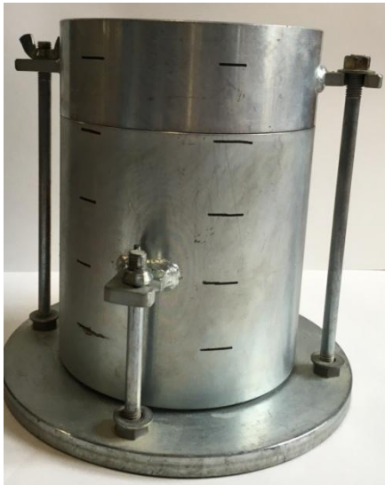
Figure 5.6. Sample preparation (a) Clay-sand mixed soils from Maizuru embankment (b) Standard proctor mould and hammer used for soil compaction
