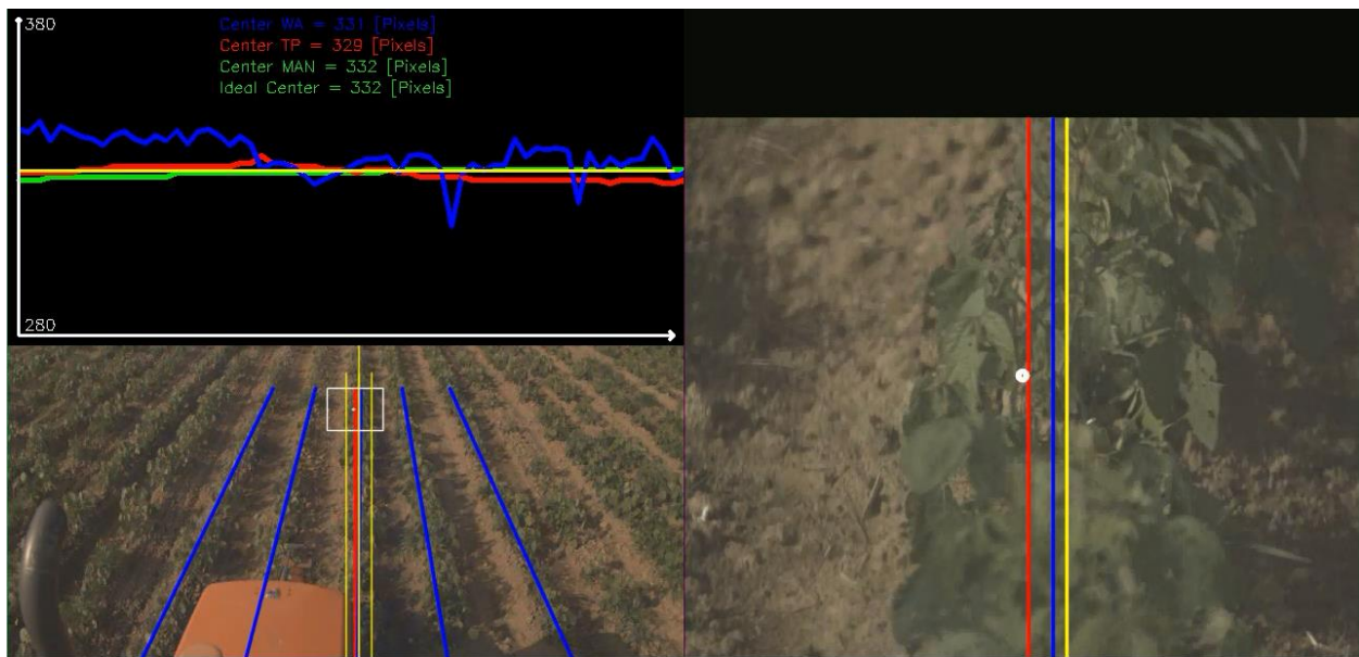
Fig. 4.19. Crop row detection detail.
