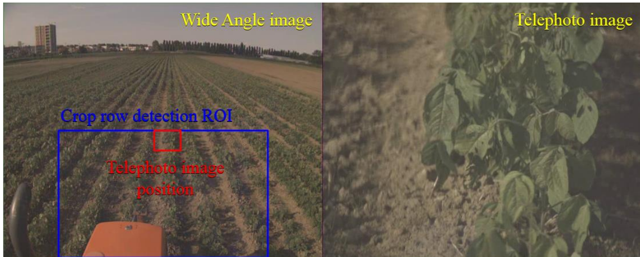
Fig. 4.17. Fujifilm 2-in-1 camera field of view; wide-angle image (left) and telephoto image (right).
