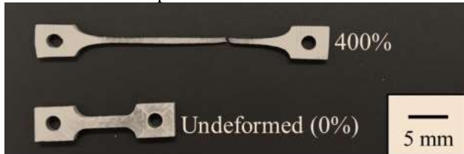
Fig. 4.12 Tensile specimens of the Mg-Li alloy without Al coating at 573 K at 0.001 \text{ s}^{-1} in the air.
