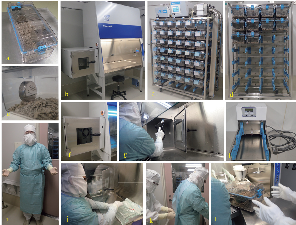
Fig. 1. Sentry Sealed Positive Pressure (SPP) cage system and personal protective equipment. a. Sentry SPP cage. b. SC-Plus Safety Cabinet. c. Rack for Sentry SPP cages. d. Sani-Rack. e. Intra-cage HEPA filter. f. Transfer chamber. g. The SC-Plus Safety Cabinet and the transfer chamber are sterilized by spraying them with soft acidic hypochlorite solution. h. SPP QDX device. i. The sterile operator wears a mask, hood, and sterile surgical gown. j. The sterile operator also wears long sterile gloves. k. The assistant wears a mask, hood, and sterile gloves, and assists the sterile operator. l. The assistant returns the changed cage from the cabinet to the rack.
