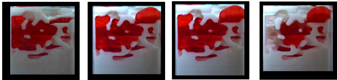
Ca = 3.0 \times 10^{-5} ( t^* = 0.54 ) Ca = 3.0 \times 10^{-3} ( t^* = 0.54 ) Ca = 3.0 \times 10^{-2} ( t^* = 0.62 ) Ca = 3.0 \times 10^{-1} ( t^* = 0.42 ) (a) Experimental results of the silicone oil in water (Case 4 in Table 5-3)
