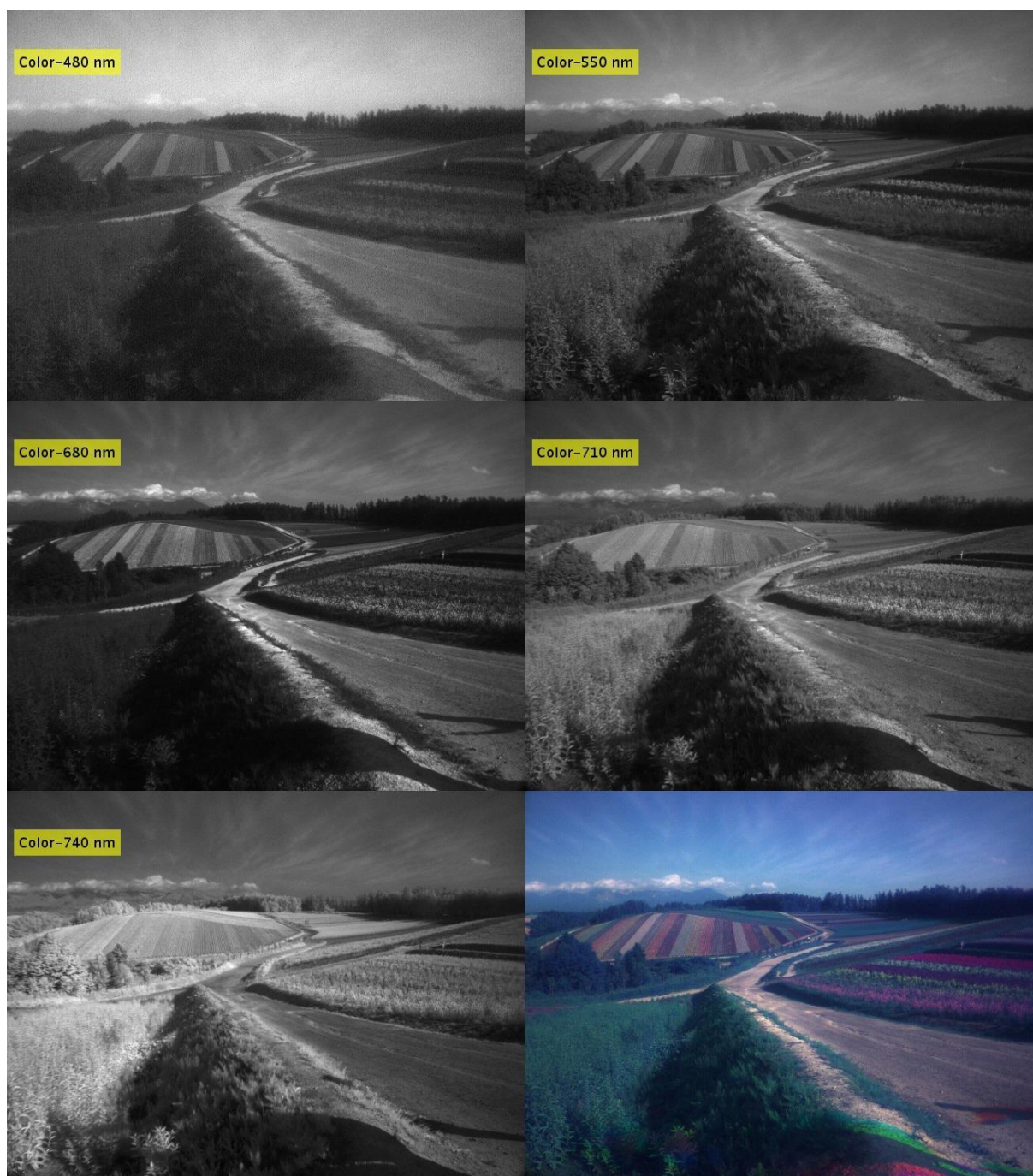
Fig. 15. Sample images of hyperspectral LCTF camera at Furano flower garden in Hokkaido, five different wavelength of images are chosen to present, and a color image is representation of Fig. 3.
