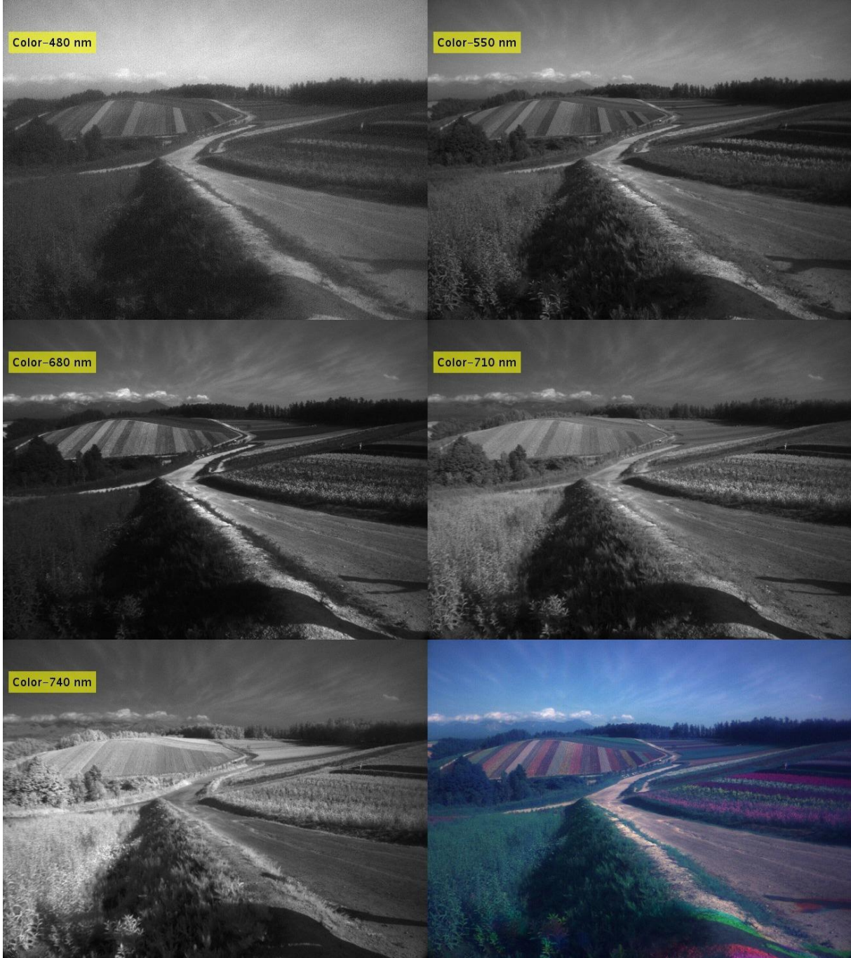
Fig. 15. Sample images of hyperspectral LCTF camera at Furano flower garden in Hokkaido, five different wavelength of images are chosen to present, and a color image is representation of Fig. 3.
