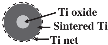
Fig. 8 Illustration of the cross-section of Ti basket after the experiment.
