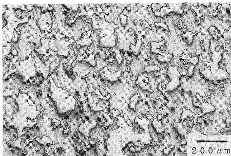
Fig. 1 Microstructure of the as-extruded compact. Copper content: 53 mass%.
