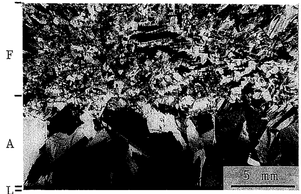
Fig. 2. Microstructure of the sample held at 1 696 K for 7.2 ks. L, A and F are liquid phase, austenitic phase and \delta -ferritic phase, respectively.
