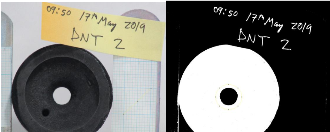
(left) setting the scale using grid paper; (right) measuring area of particles at throat
