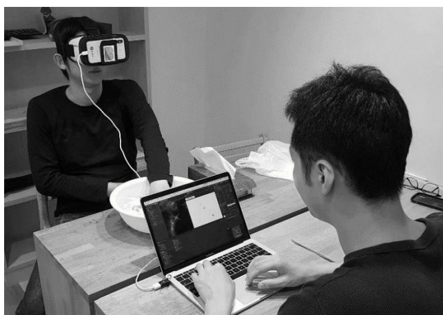
Figure 2-3. Experiment setup including Smartphone based VR-HMD, controller PC, water with ice in wash ball.
