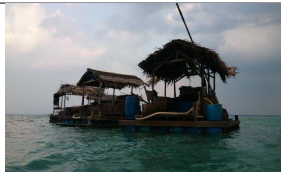
Small-scale coastal tin mining pontoon operating in Tanjung Gunung Waters (Field Research, Tanjung Gunung, 2014)
