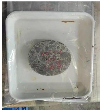
Fig.1.4 The set up of the water absorption test
