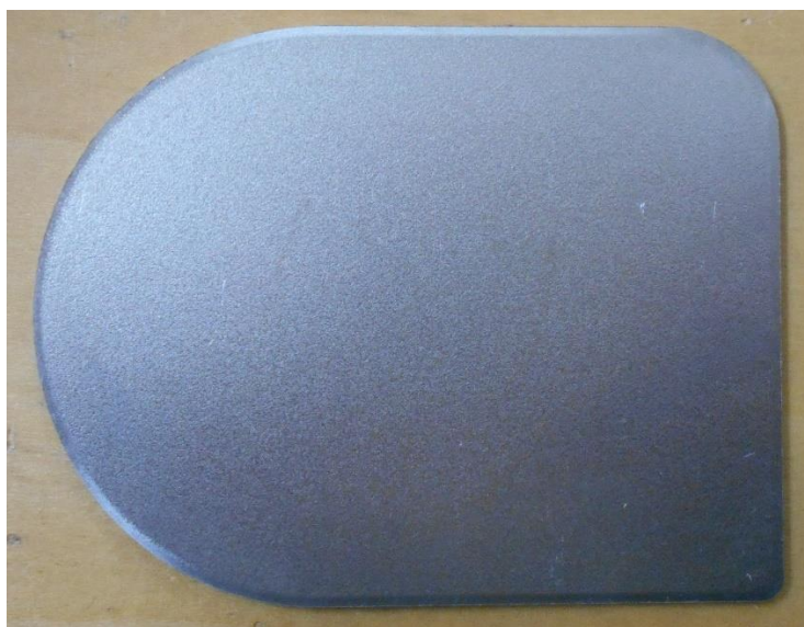
Fig. 5.4 The processed product obtained by the blanking testing.
