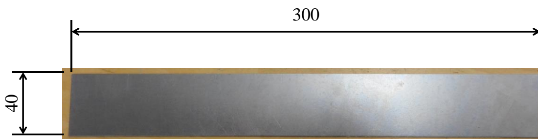
Fig. 3.2 Geometry of tensile test specimen.
