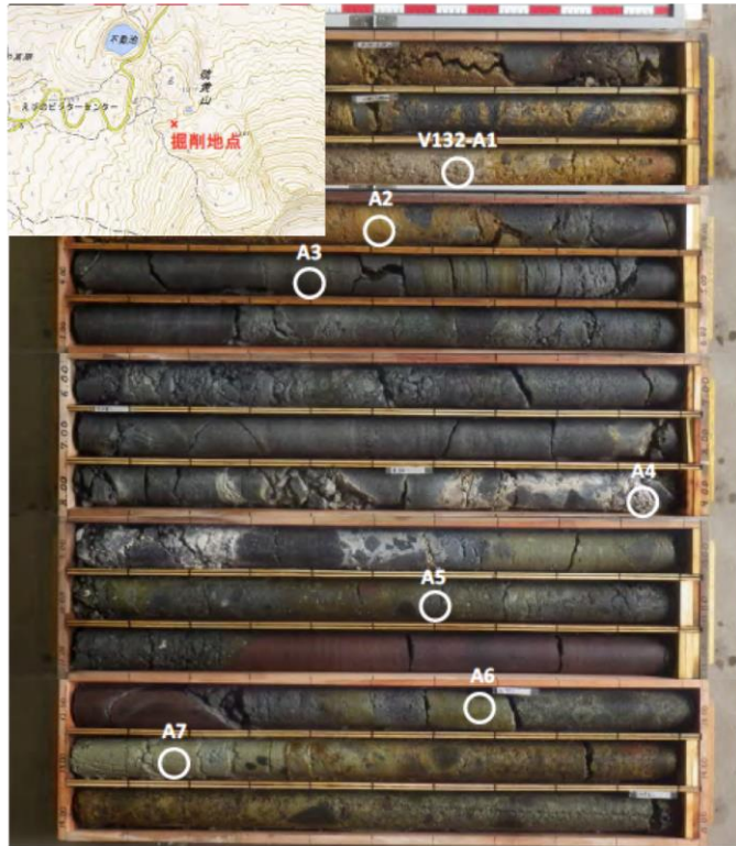
Fig. 2.6.5 (a) Drilling core at 1km west of Iwoyama. Drilling depth is 400 m. There are alternately soft (軟石) and solid rock faces. (b) Drilling core at 300 m south of Iwoyama. Drilling depth is only 15 m. A1-A3 correspond to deposit of edifice collapse of Mt. Karakuni-dake. A4-A6 correspond to deposit of ash and block from Mt. Karakuni-dake. A7 corresponds to deposit of Kobayashi pumice.
