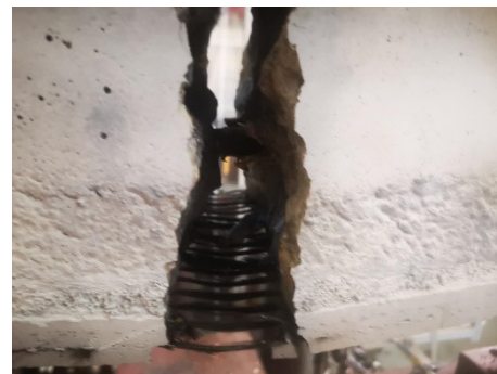
(e) Carbon-FRCM failure in C-B-L4-F70
