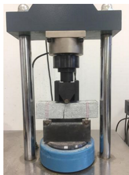
(a) Flexural strength testing
