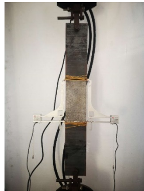
Fig. 2.16 Tensile tests setup of carbon-FRCM specimens.
