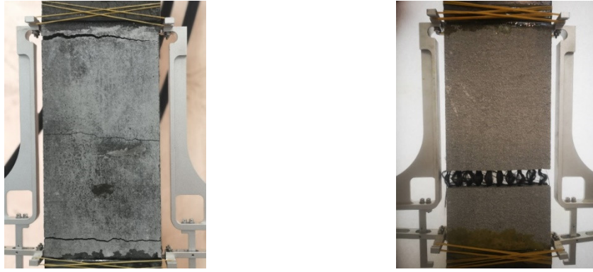
(a) Tensile failure mode under static loading (b) Tensile failure mode under cyclic loading Fig. 3.3 Comparison of tensile failure modes of carbon-FRCM under static and cyclic loading.
