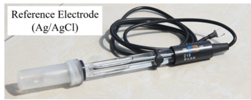
(a) Ag/AgCl reference electrode
