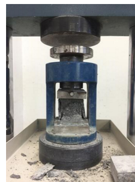
(b) Compressive strength testing
