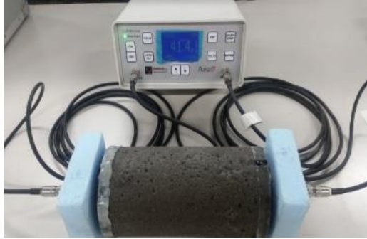
Figure 3.3: Ultrasonic pulse wave velocity setup
