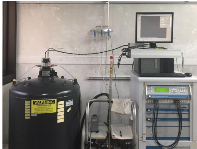
Fig. 2.9 Picture of the PPMS-9T in NIMS Namiki-site
