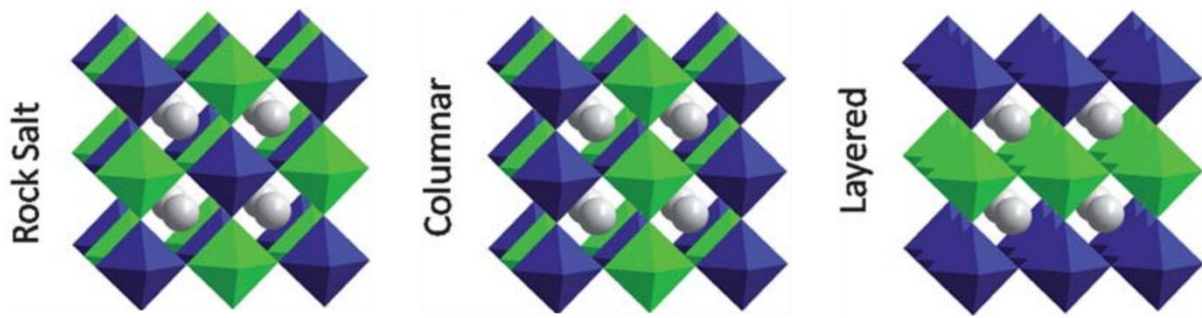
Fig. 1.3 B-site ordering schemes in double perovskites A_2BB'O_6 [14]
