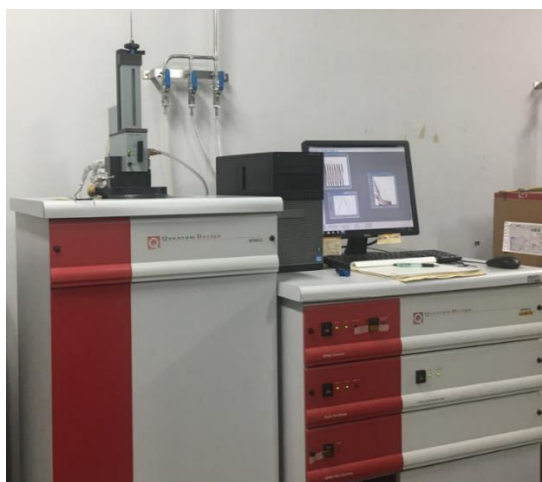
Fig. 2.8 Picture of the MPMS-7T in NIMS Namiki-site
