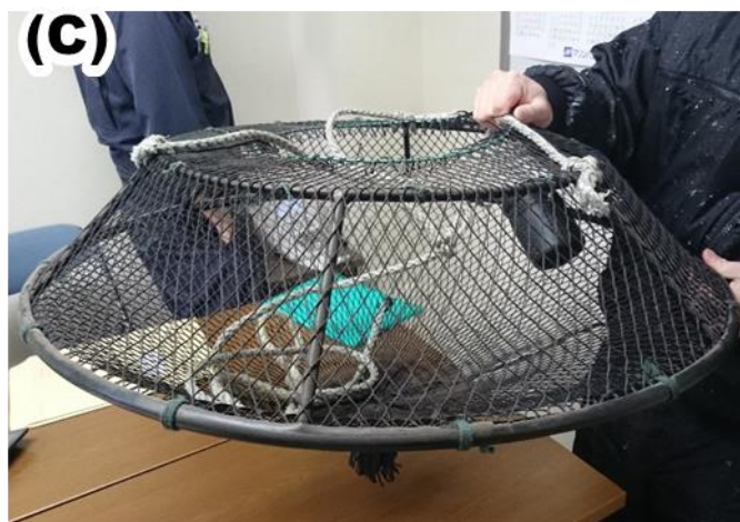
Fig. 5-2. The overview apparatus for exterminating of sea stars, the dredge net (A), star mop (B) and star pot (C).
