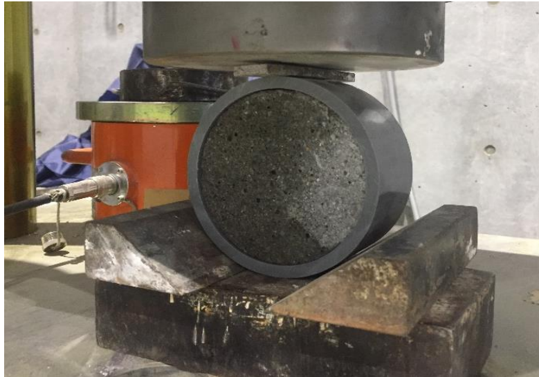
Fig. 2.3: The specimen subjected to splitting load
