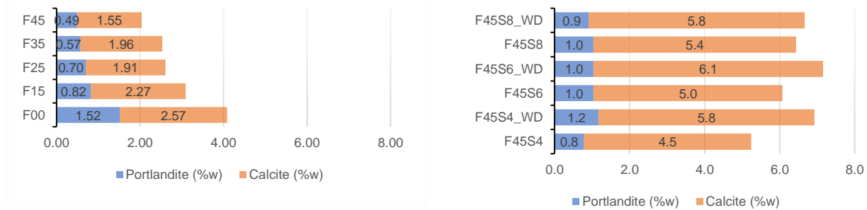
Fig. 2.16: Thermogravimetric analysis results [mass%] for portlandite content and calcite content
