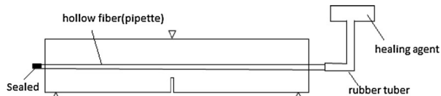
Fig. 1.5: Testing diagram of external healing agent supply system [10]
