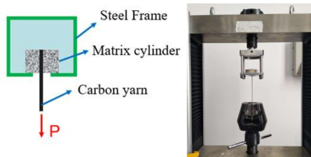
Fig. 2.1 Test setup for pullout tests
