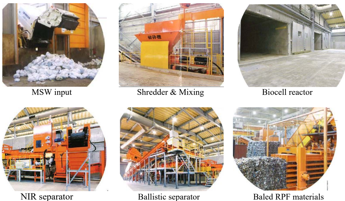
Figure 3-3 Images of process flow in Biomass Resource Center Mitoyo referred from the pamphlet
