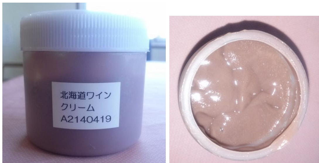
Fig.4 Picture of test specimen cream with GSE (Day 0) (Extracted condition: 80% ethanol, for 2 h at 60 ° C).
