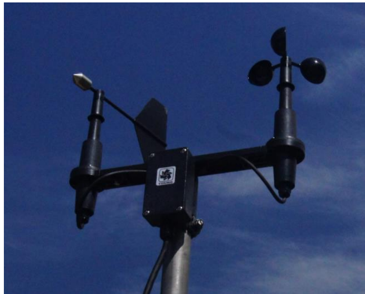
Figure 3.7 Wind speed and wind direction sensors.
