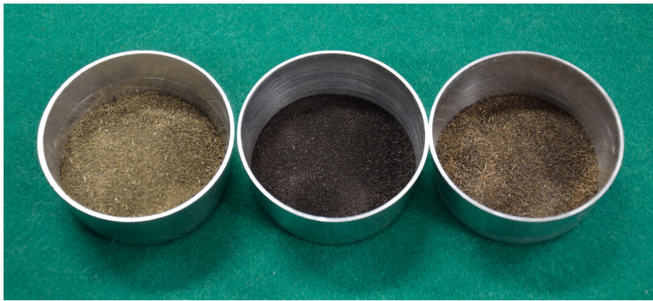
Fig. 2.4 Appearance of raw dairy manure (left), the manure prepared under air at 90 °C (center), and the manure treated under N 2 at 90 °C (right). All samples were dried before photographs were taken to eliminate the effect of water on the color.
