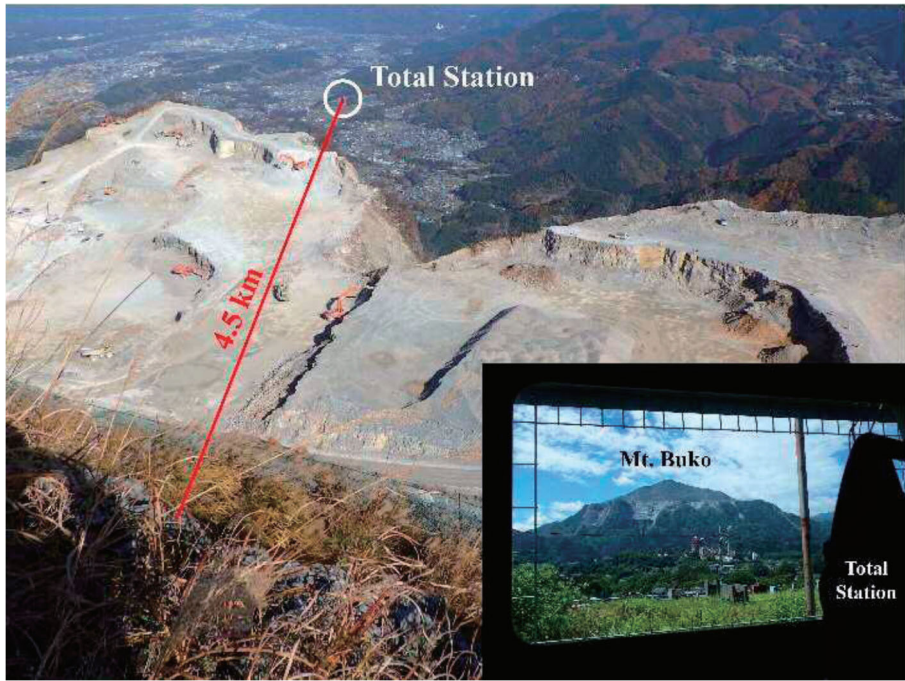
图 2 - 6 The line of the sight of APS and a view of Mt. Buko from the Total Station 8) .
