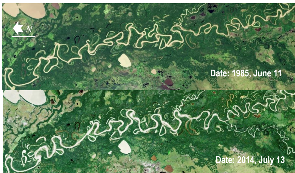
Figure 1.1: Changes in the meander migration pattern observed along 28 years for the Mamore river in Bolivia. NASA Earth Observatory images by Jesse Allen, using Landsat data from the U.S. Geological Survey. Caption by Kathryn Hansen
