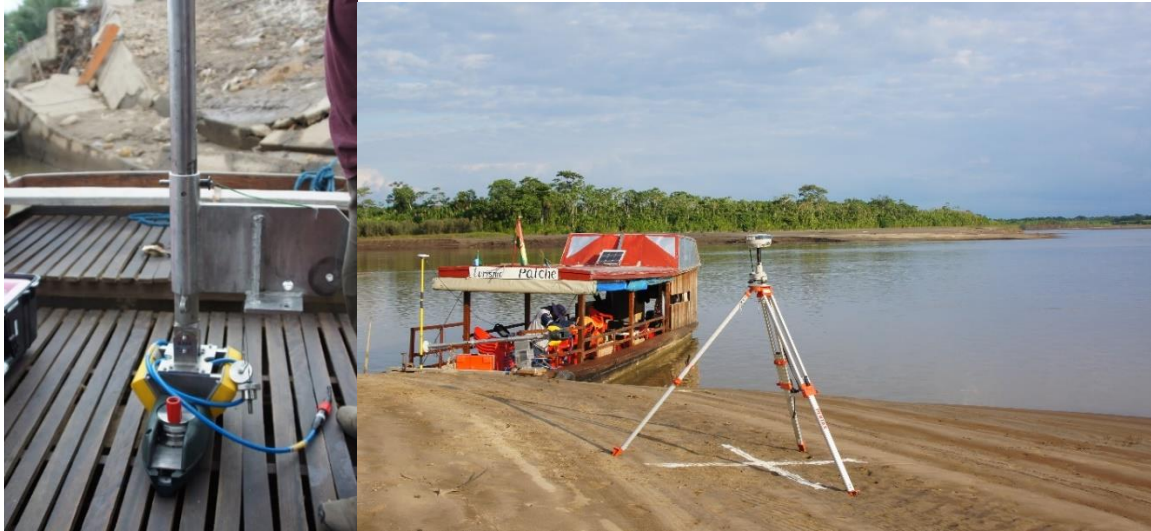
Figure 3.1: MBES equipment installation (left) during field surveys in the Ichilo and RTK GPS (right) used during the field surveys.
