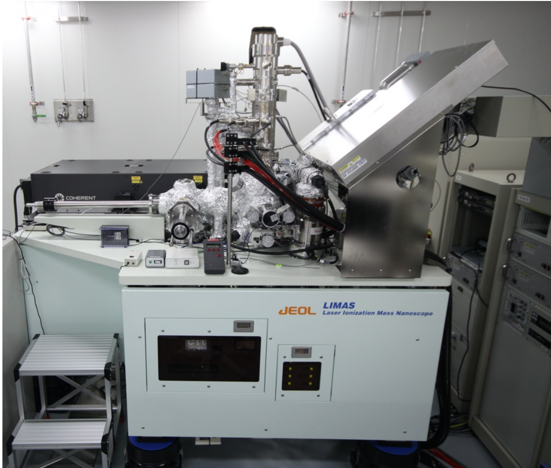
Figure 1: Photograph of isotope nanoscope (Laser ionization mass nanoscope, LIMAS).
