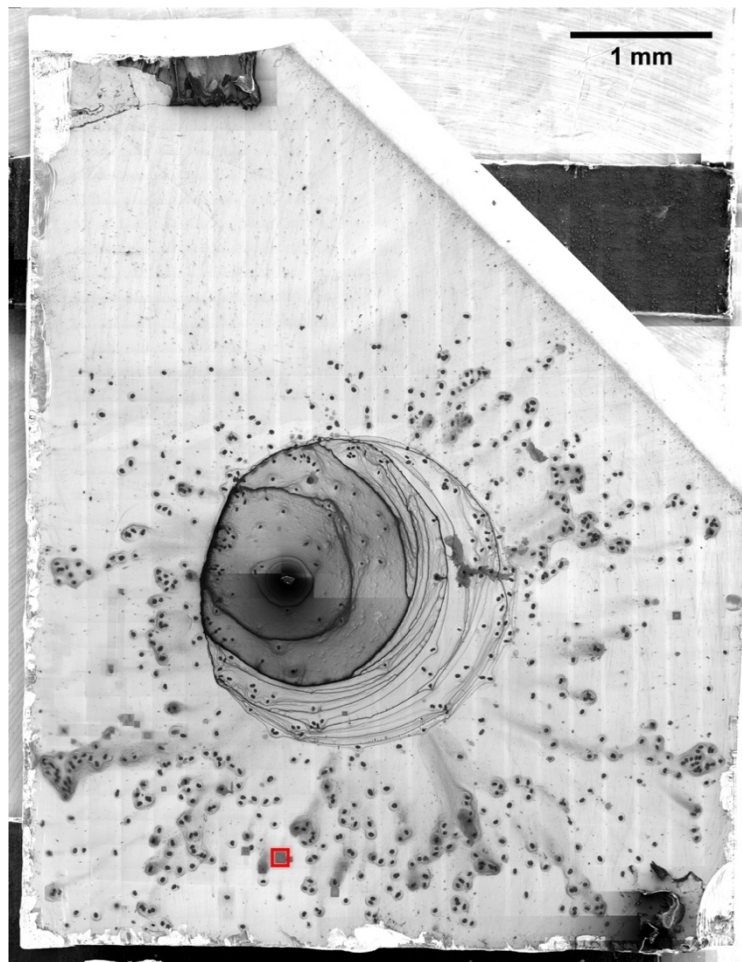
Figure 13: Secondary electron image of chromosome spreads dropped on Si wafer substrate. A chromosome spread marked by red square is shown in Figure 14.
