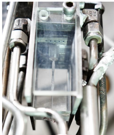
(b) Inside of the duct with a fuel sample installed.
