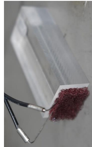
Fig.2.2 Picture of a fuel sample with ignition apparatus.
