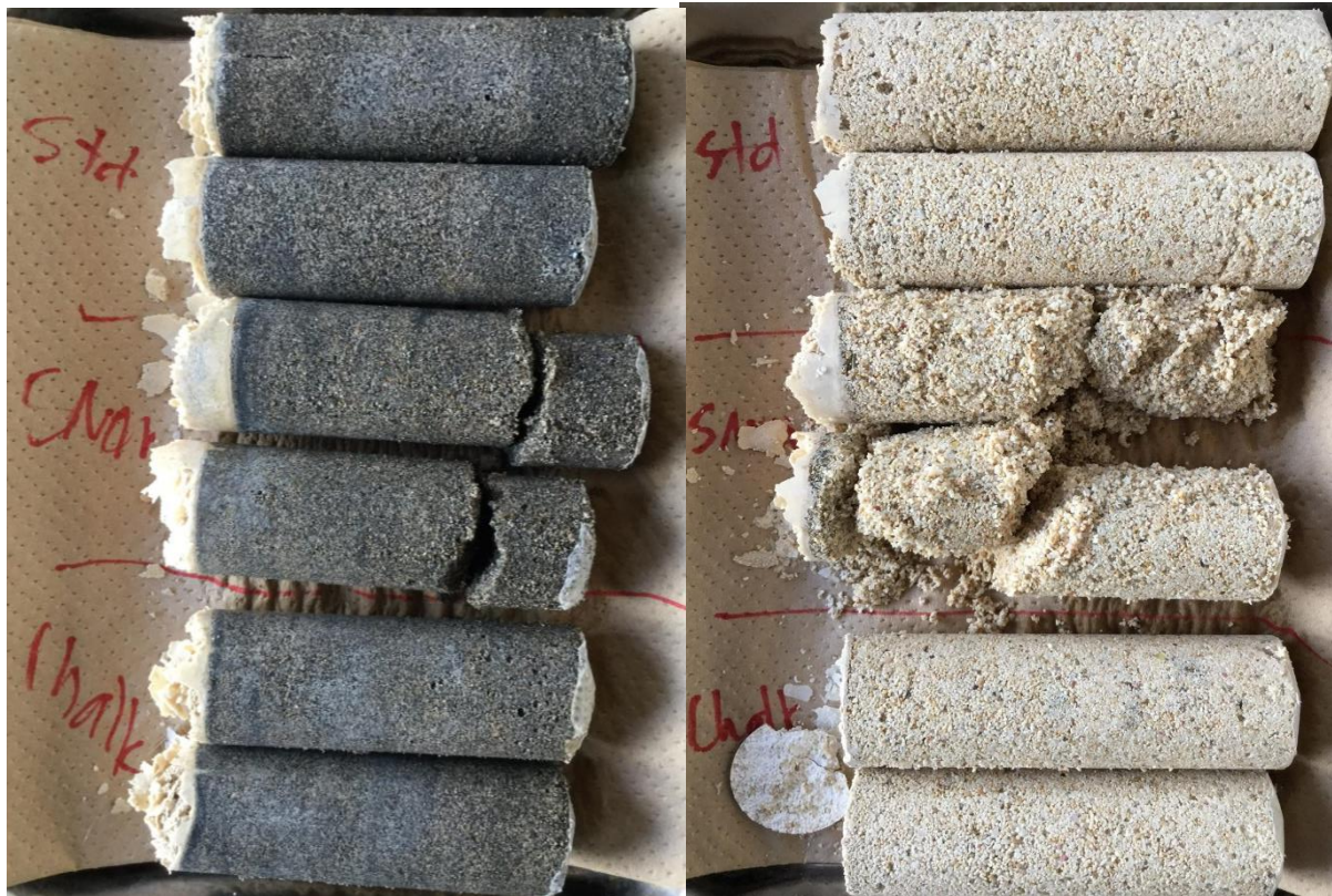
Figure 7.6 Beach sand treatment test using microbial induced carbonate precipitation after 14 days treatment. Sample with nigriscent color (left) is Quartz silica sand from Parangtritis beach and sample with whitish color (right) is carbonate coarse sand from Krakal-Sadranan beach sand.
