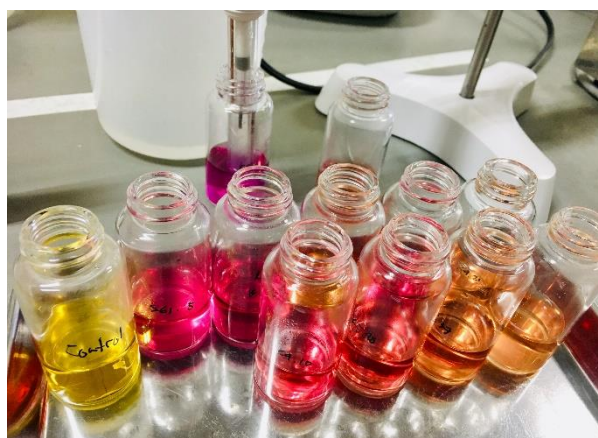
Figure 5.2. Appearance of discoloration of the urease activity measurement solution (yellow is neutral, purple is alkaline).
