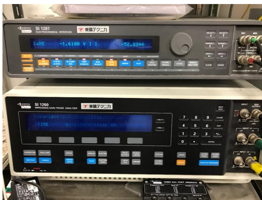
Figure 2-4 The solartron 1260A frequency response analyzer implemented with a Solartron 1287 potentiostat.
